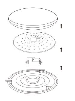
• Please ensure no any metal is thielding the sensor antenna.
